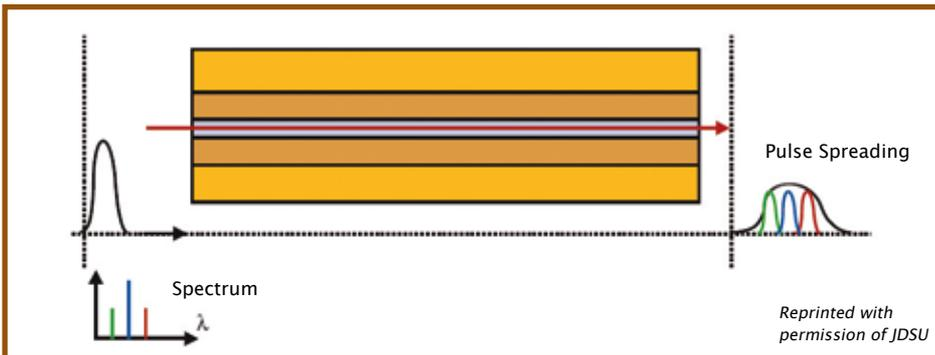
When we transmit light into the fiber, we usually talk about transmitting at one wavelength, 1310nm or 1550nm. But in fact our light source, (usually) transmits at several wavelengths, 1548, 1549, 1550, 1551, and 1552nm. When optical signals are transmitted through the fiber, the different wavelengths travel at different speeds. This is what we call chromatic dispersion.
