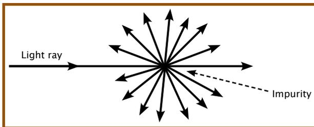
As light travels through the fiber, it hits impurities. These impurities will cause the light to reflect in many different directions, giving a loss.
