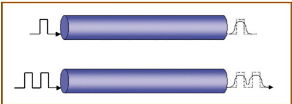
In the first picture we can see that the signal is degraded as it travels through the fiber. The longer the fiber, the more flattening of the pulse. On the lower picture we can see two pulses. Notice, on the right hand side, that there is a problem distinguishing the one pulse from the other. This is called dispersion.
