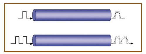
In the first picture we can see that the signal is degraded as it travels through the fiber. The longer the fiber, the more flattening of the pulse. On the lower picture we can see two pulses. Notice, on the right hand side, that there is a problem distinguishing the one pulse from the other. This is called dispersion.
