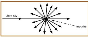
As light travels through the fiber, it hits impurities. These impurities will cause the light to reflect in many different directions, giving a loss.
